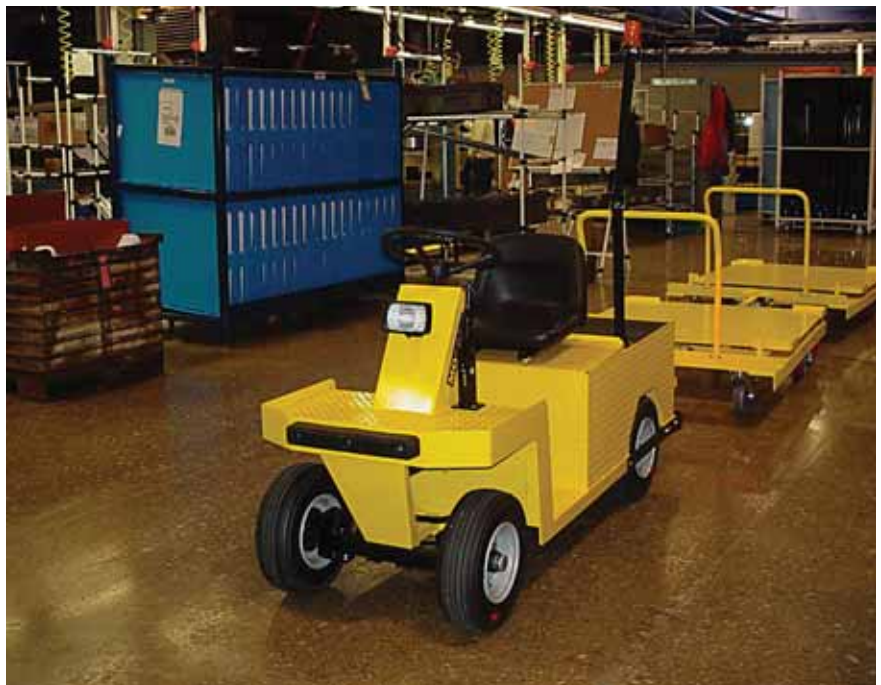
Instead of using forklifts to deliver parts to the line, the company opted for a system of carts pulled by electric tuggers. Photo courtesy Kinetic Technologies
