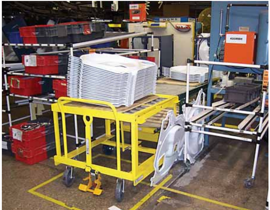
Boxes of parts are presented to the line on in-and-out flow racks custom-built from modular hardware. Photo courtesy Kinetic Technologies
