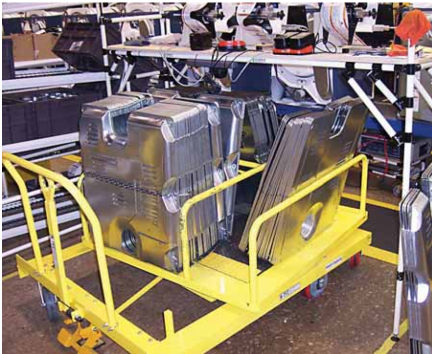
Metal stampings are delivered to the line on carts with bases that rotate 360 degrees. Photo courtesy Kinetic Technologies
