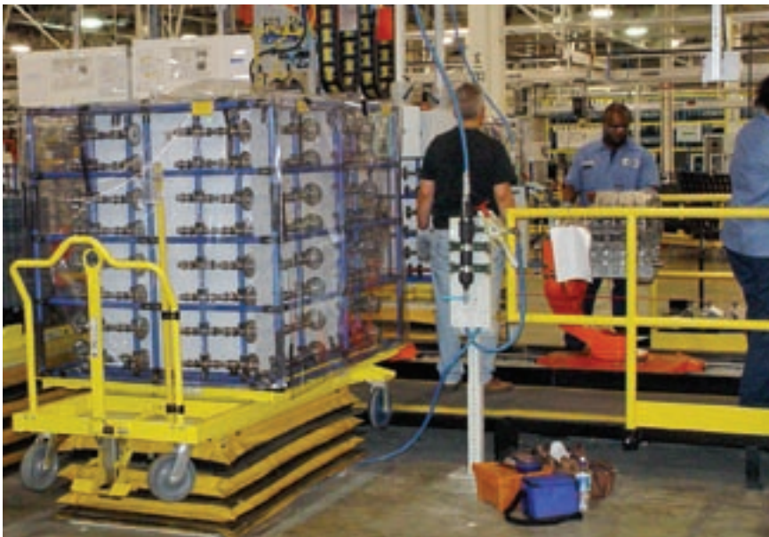
The use of rotating upper frames and under frame lifts helps to prevent worker injuries when working from carts.
