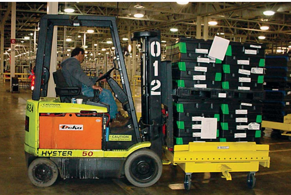
Forklifts are confined to the dock, where they transfer skids of parts from trucks to the carts. Photo courtesy Kinetic Technologies
