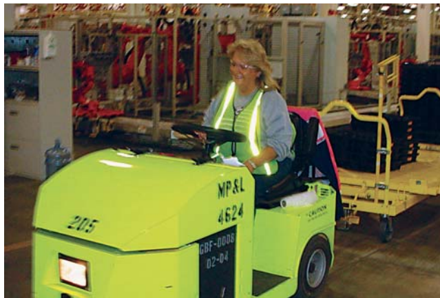
Parts are delivered to the line in bins or custom-built racks traveling on wheeled carts pulled by electric tuggers.
