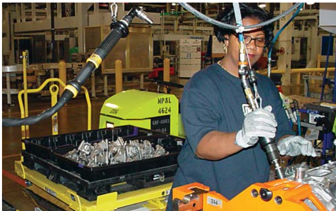
Using carts to deliver parts to the line has saved space. Because parts can be sequenced and loaded onto racks at a central location, there's less need to store all the parts for different engine models on the line.
